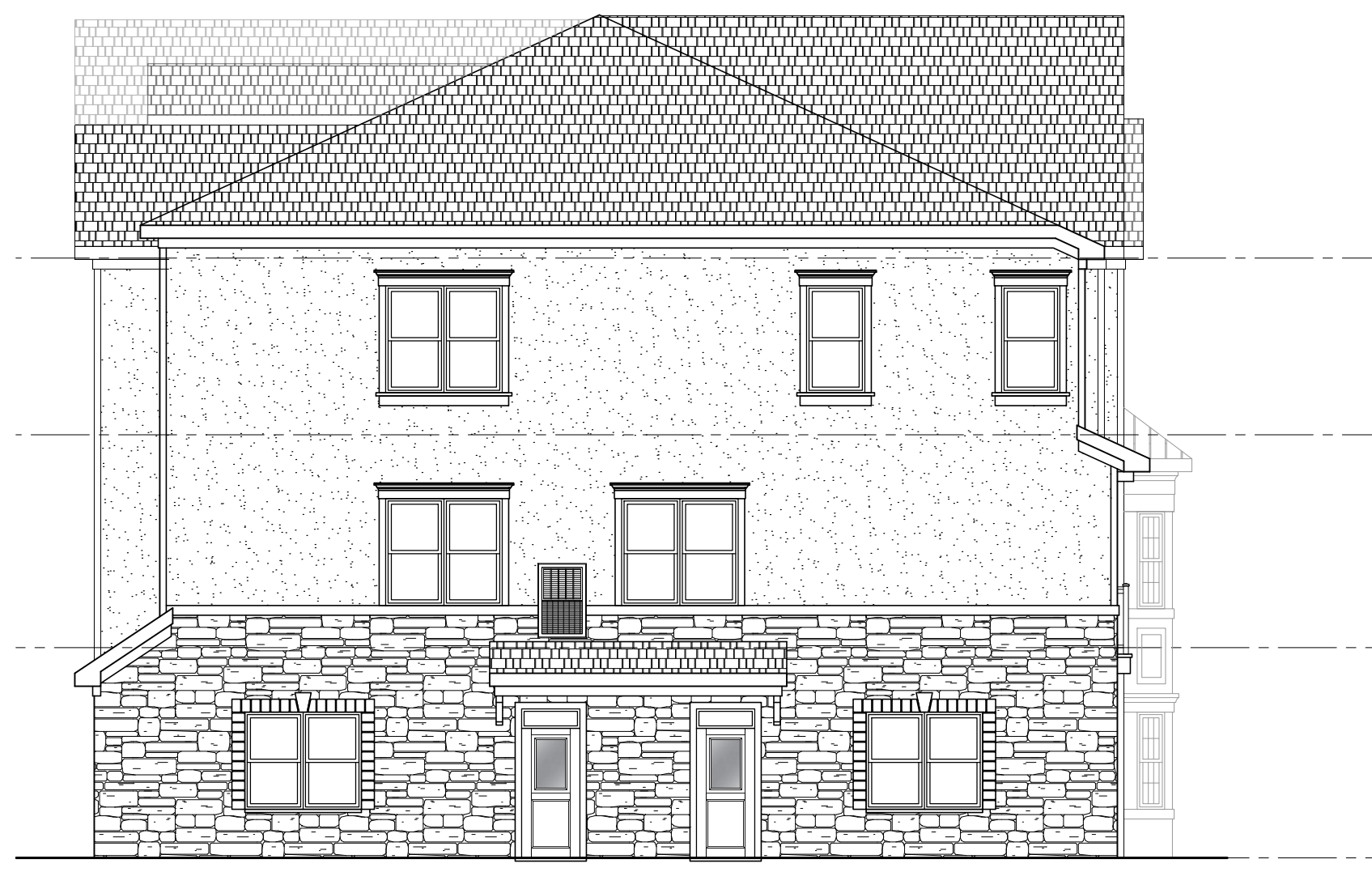
4 BUILDING A - SIDE ELEVATION BLDGS: 3, 5, 9, 15, 16, 21 SCALE: 1/8" = 1'-0"
