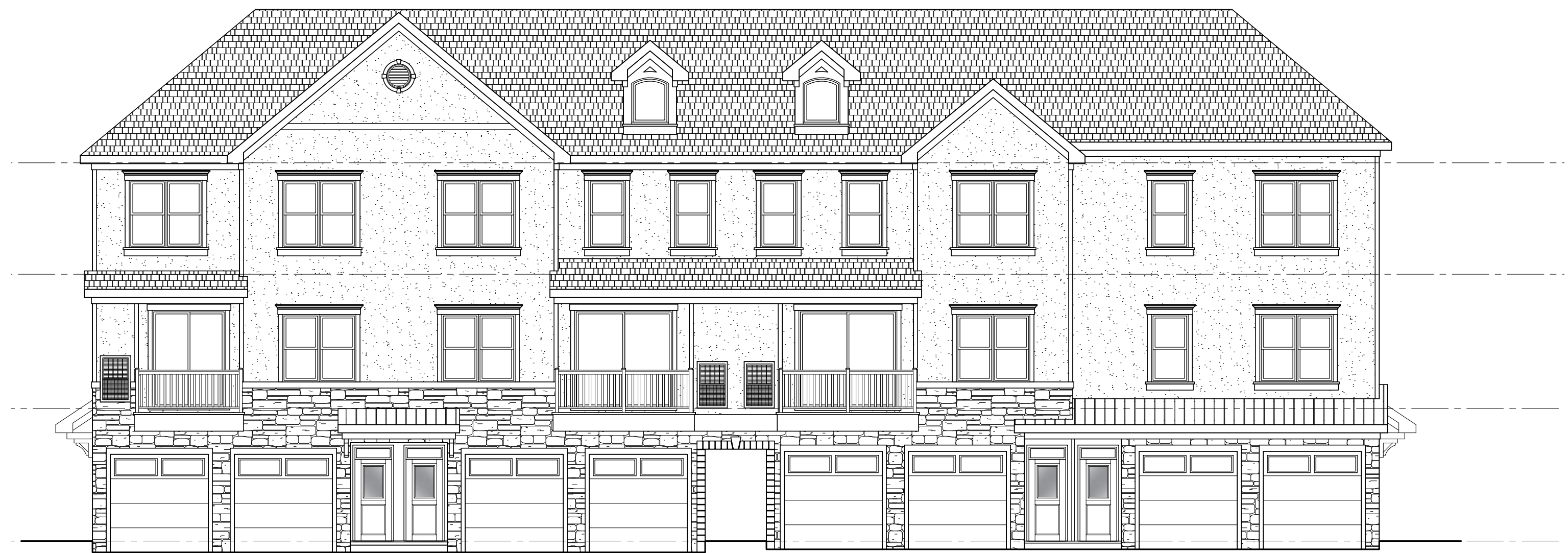
2 BUILDING A - GARAGE ELEVATION BLDGS: 3, 5, 9, 15, 16, 21 SCALE: 1/8" = 1'-0"
