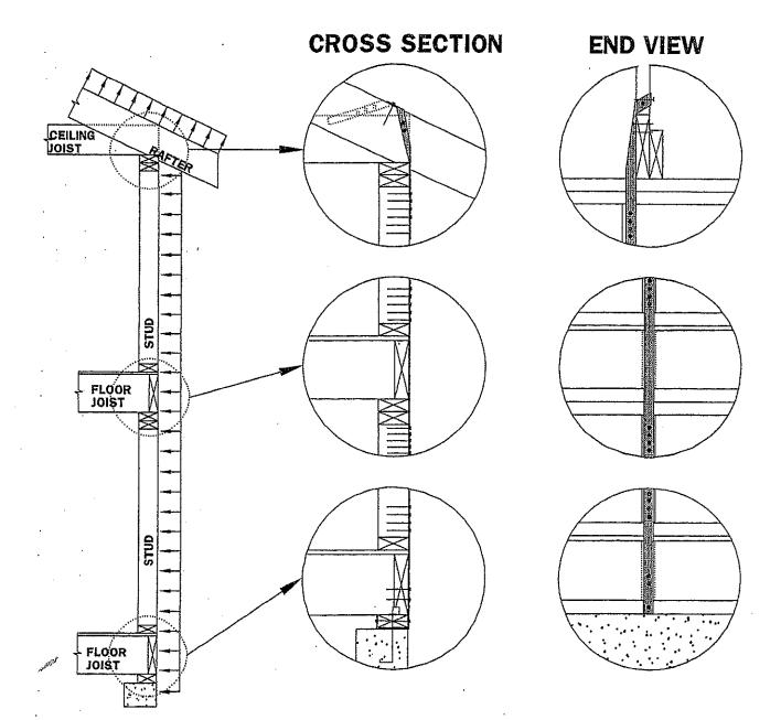
Figure 2.2a Typical Lateral Framing Connections
