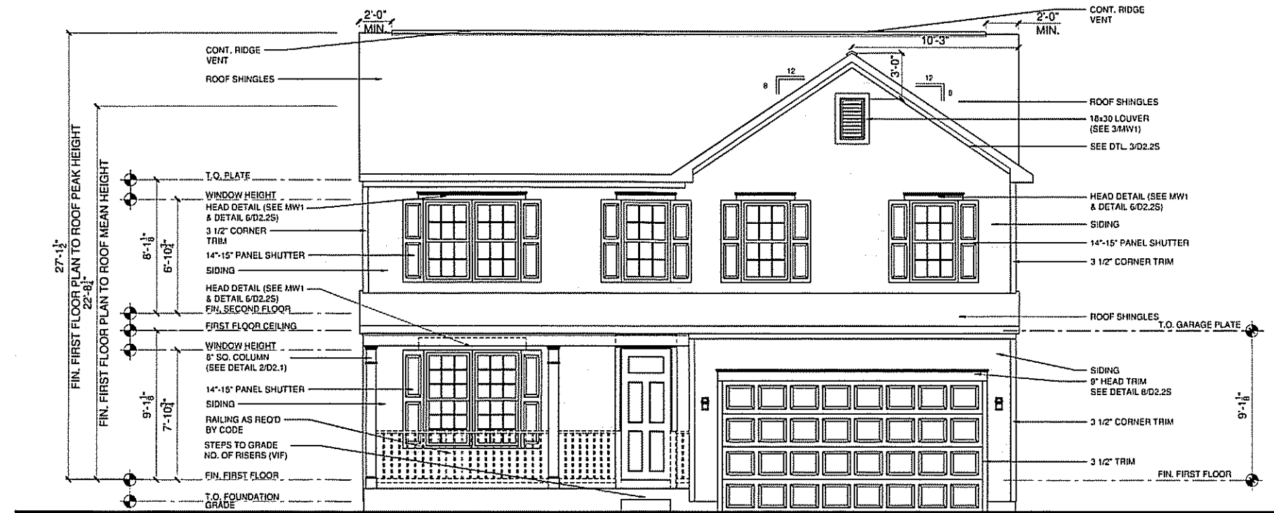
1 FRONT ELEVATION - FORM 'C' (SIDING)
