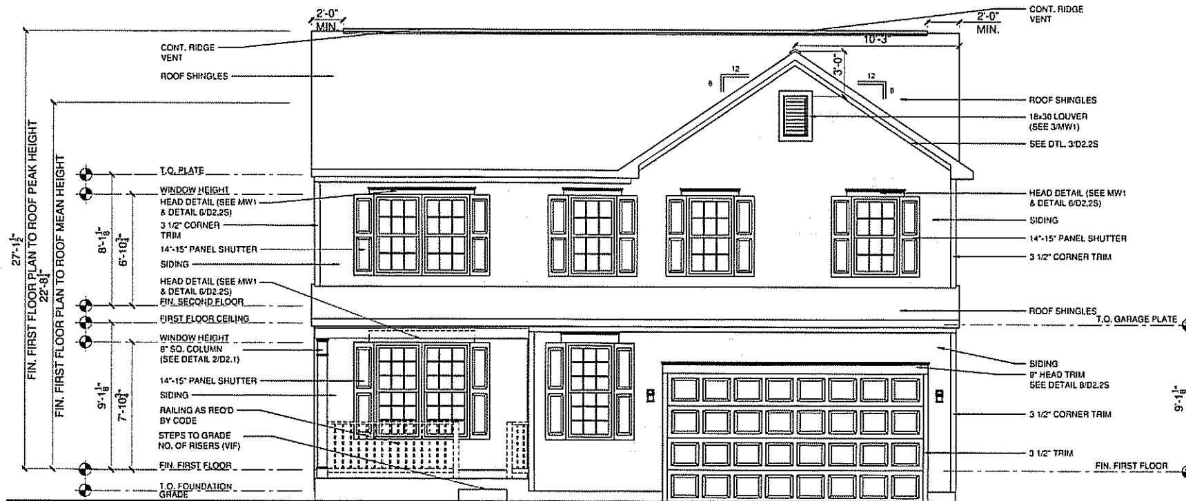
1 FRONT ELEVATION - FORM 'C' ALTERNATE ENTRY (SIDING)
